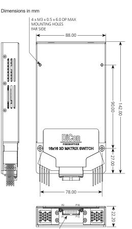
MATING CONNECTOR P/N: TCSD-08-01-F-N SAMTEC CONNECTOR P/N: STMM-108-02-G-D
